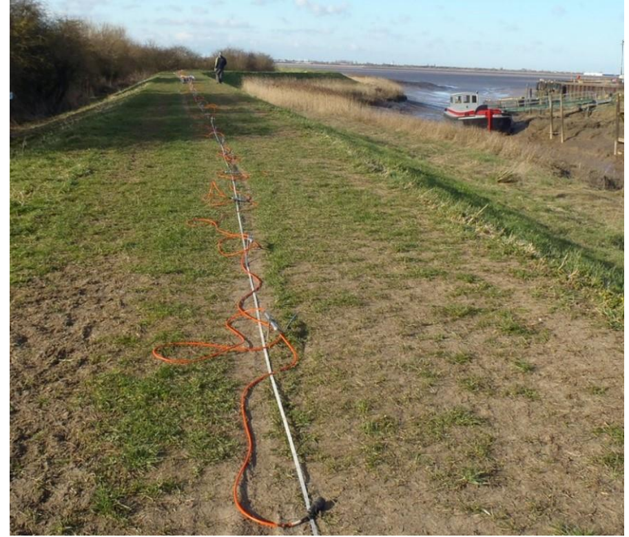
Specialist equipment being used on site including electro-magnetic profiling (left) and electrical resistivity tomography (right)
