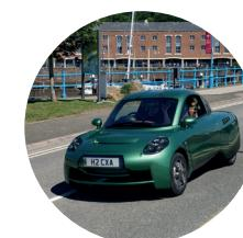
The Riversimple Rasa is powered using a hydrogen fuel cell, which utilises a chemical reaction between hydrogen from the Rasa hydrogen tank and oxygen from the air to produce electricity on board the vehicle.
