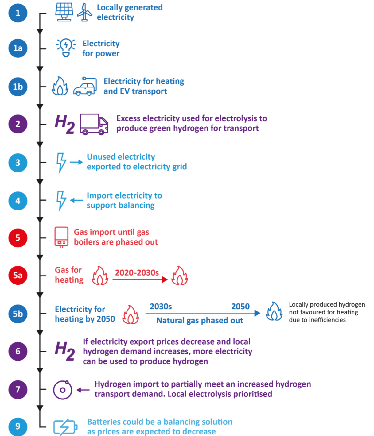
Figure 28: Hierarchy of energy supply-demand relationship based on a 2020 world view and short-term actions to support reaching net zero by 2050
