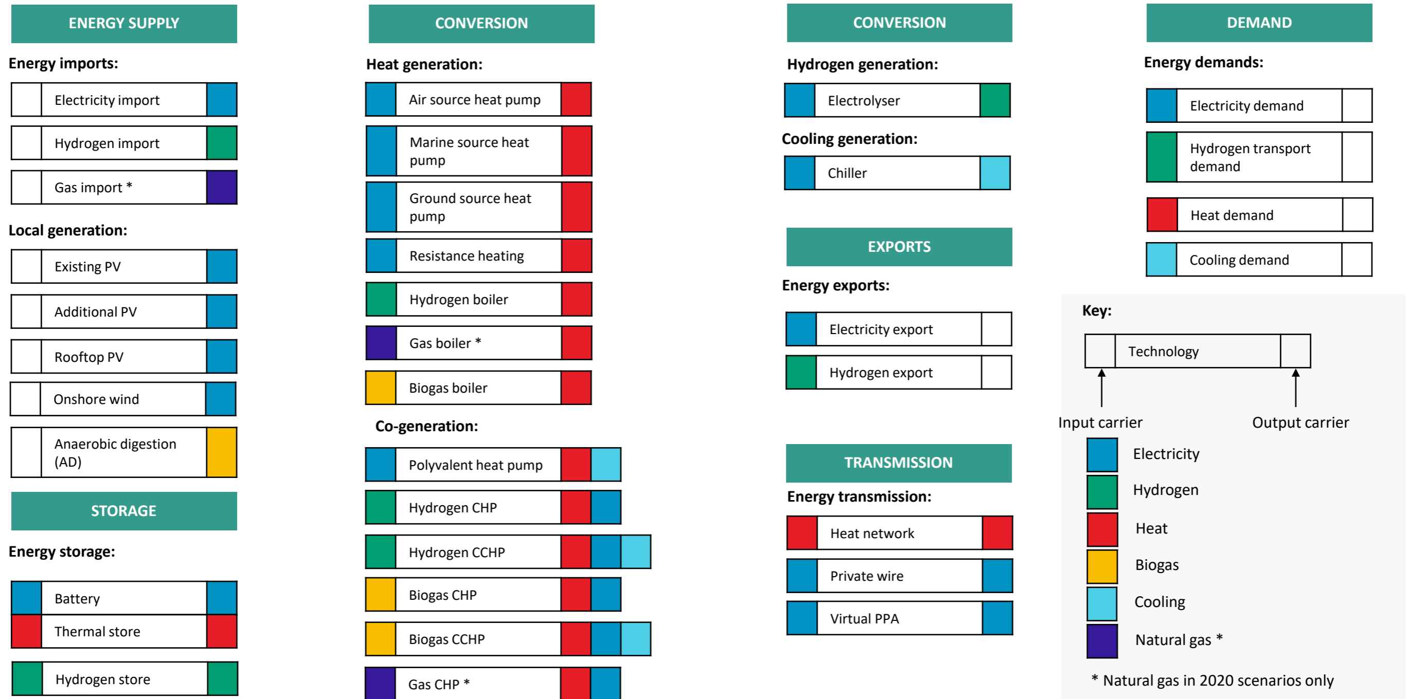
Figure 38: Complete list of available technologies across propositions highlighting their input and output energy vectors
