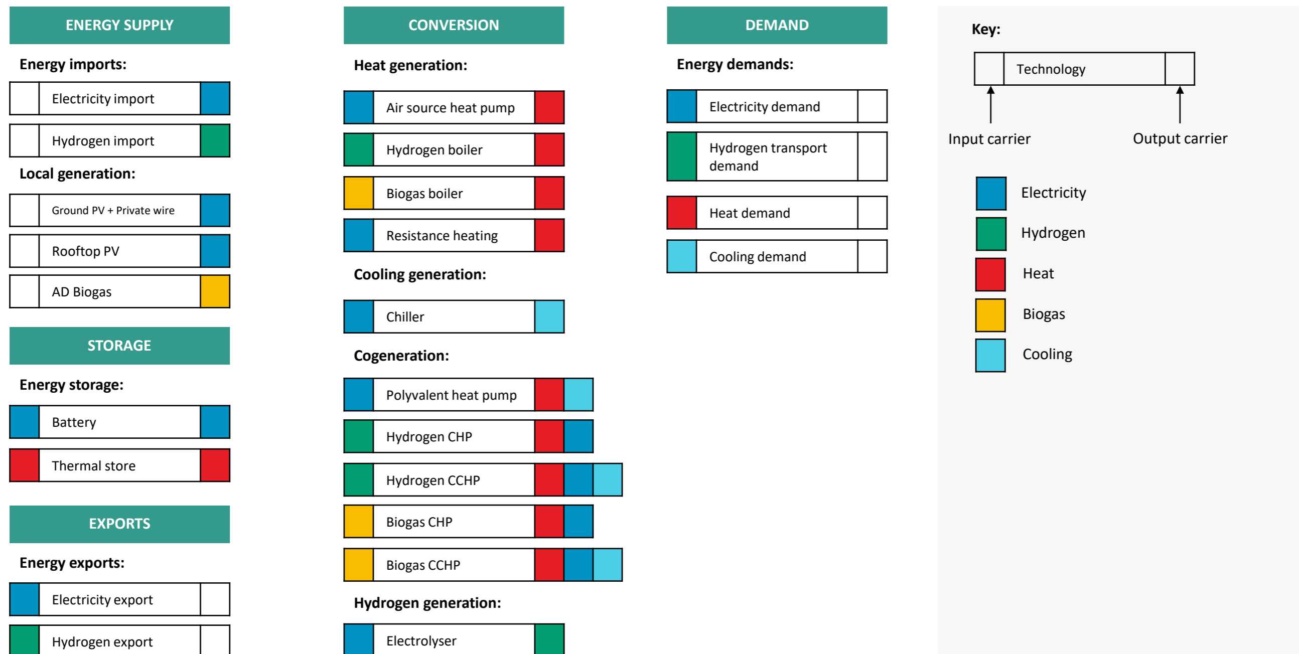
Figure 46: List of technologies modelled in Proposition 2 and their input and output energy vectors
