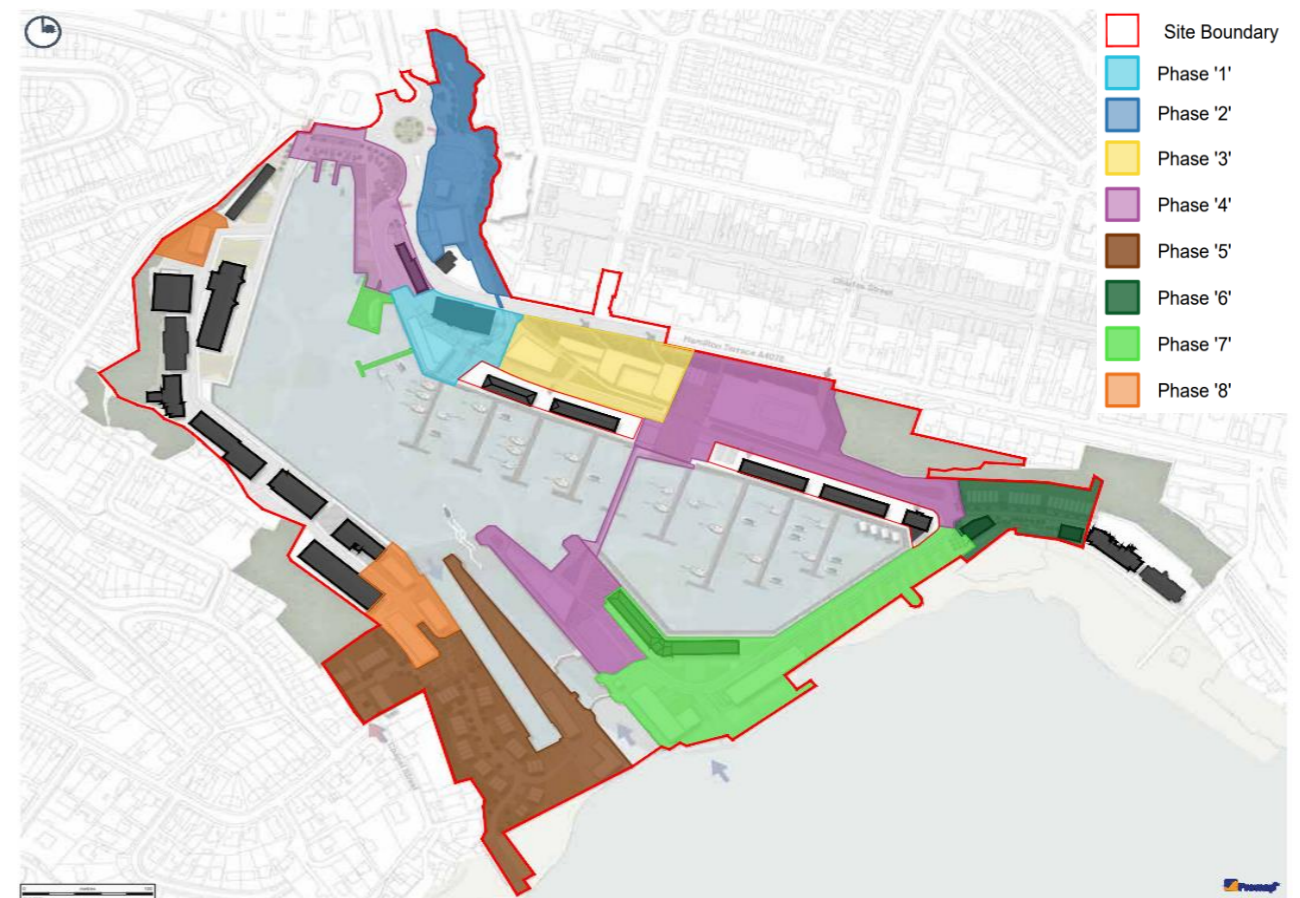
Figure 20: Site map of the proposed building phases of the Milford Haven Marina [6]
