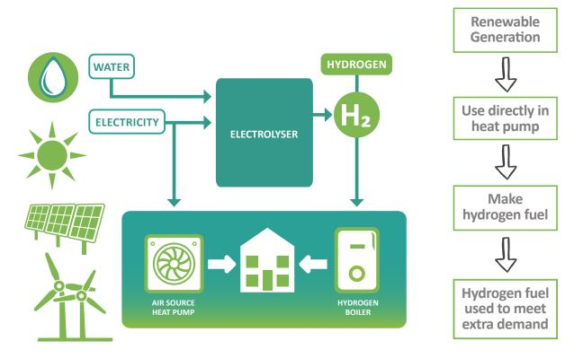
The building's heating uses renewable energy to power a heat pump. The heat pump makes use of warmth in the outside air to create a comfortable temperature inside the building. This is even more efficient than using standard electric heaters. On very cold days a heating boost is provided by a hydrogen fuel boiler.
